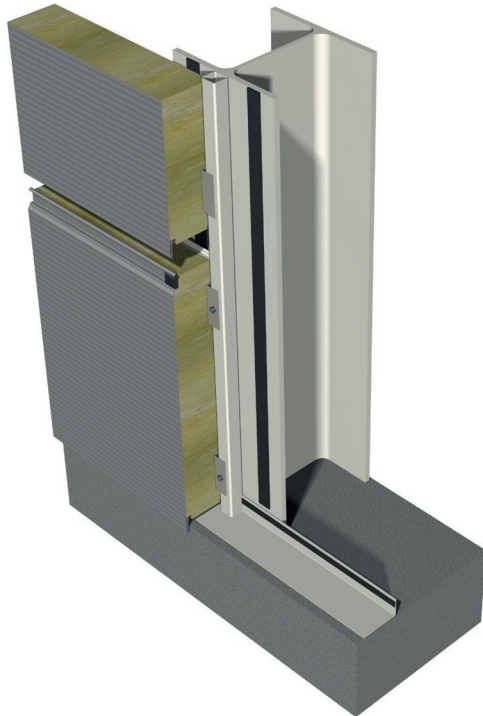
Fig. 34: Indirectly fixing back steel sheet into spacer
